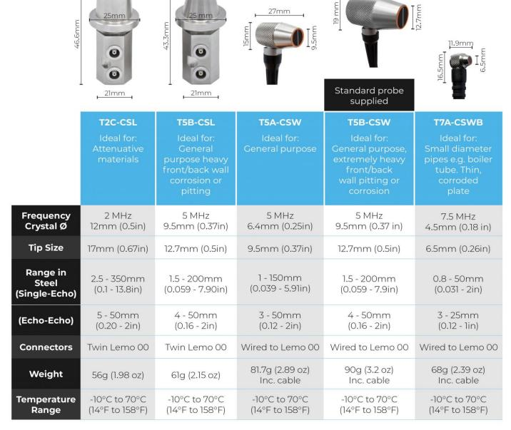
All above probes have composite crystal and need to be used with Ultrasonic Couplant when taking measurements (excl. underwater)
