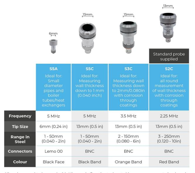
All probes need to be used with Ultrasonic Couplant when taking measurements (excl. underwater)
